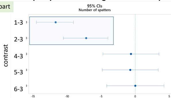
only lack-of-fusion condition (energy density 1 and 2) can be distinguished
