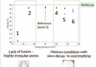
The spatial signature of spattering (via **k-functions**) allowed us to detect **all the departures** from the optimal condition
