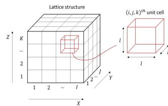
Lattice – a regular grid of unit cells
