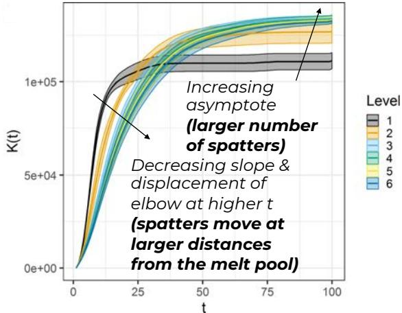
Superimposition of spatters ejected in one layer for each energy density level
