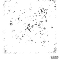
Example of porosity structure in x-ray CT scan
