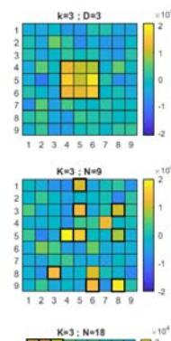
Only the Z-index can detect randomly sparse anomalies of the cooling profiles
