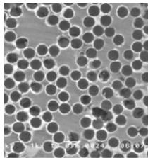
Example of CFRP
